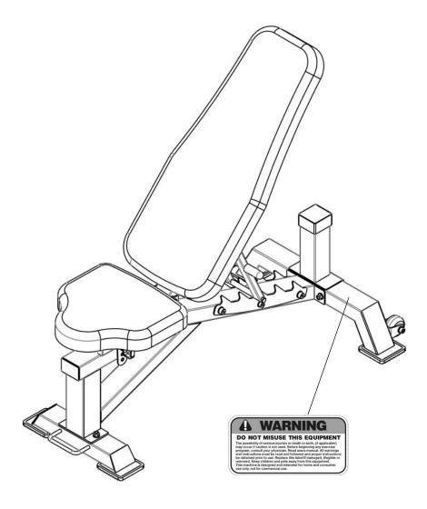
The warning labels shown here have been placed on the Rear Base. If the labels are missing or illegible, please call customer service at 1-800-999-8899 for replacements. Apply the labels in the location shown.
